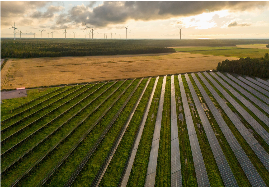
Picture 1: by Ville Suorsa/Image bank of the Ministry of the Environment in Finland Agrivoltaics installation combining solar panels with agricultural production, illustrating how renewable energy generation can be integrated with continued food production and other land-use interests.
