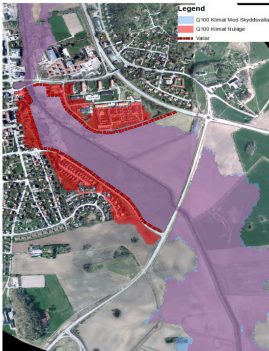
Figure 3 Map over Flood protection in Getinge, where the red striped line symbolises the sand banks, the shaded red colour symbolises the previous flooded areas and the shaded purple colour symbolise the areas that will be partially flooded after the sand banks are built.
