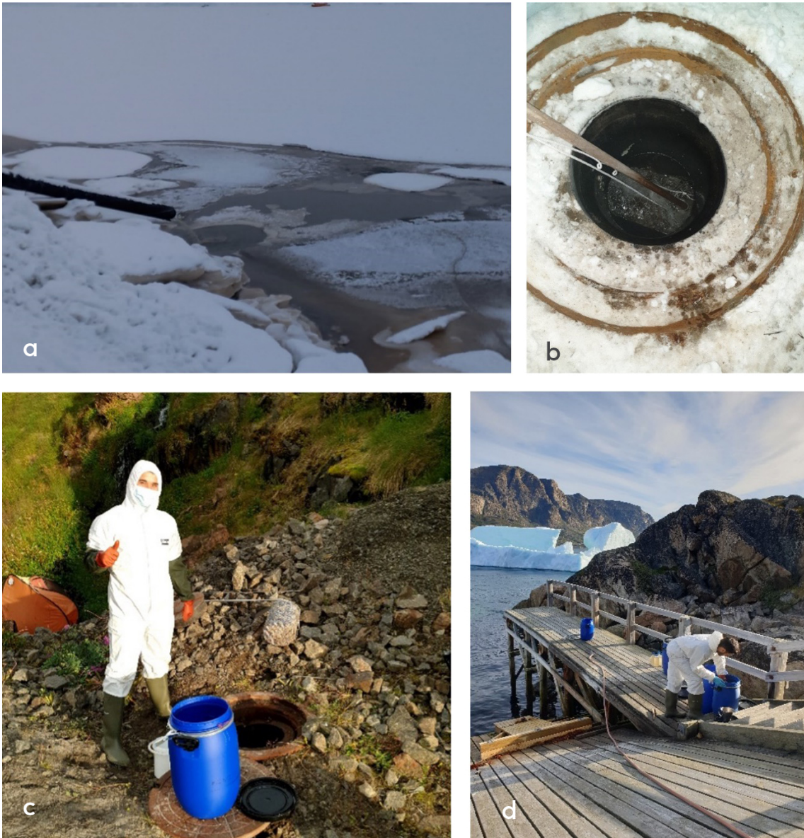
Figure 2 a) Wastewater outlet U1 in Sisimiut, March 2022, b) Sampling of macroplastics, c) Sampling of meso-plastic, d) Cleaning of meso-plastic and macro-plastic samples in Sisimiut. Photos: Pernille E. Jensen
