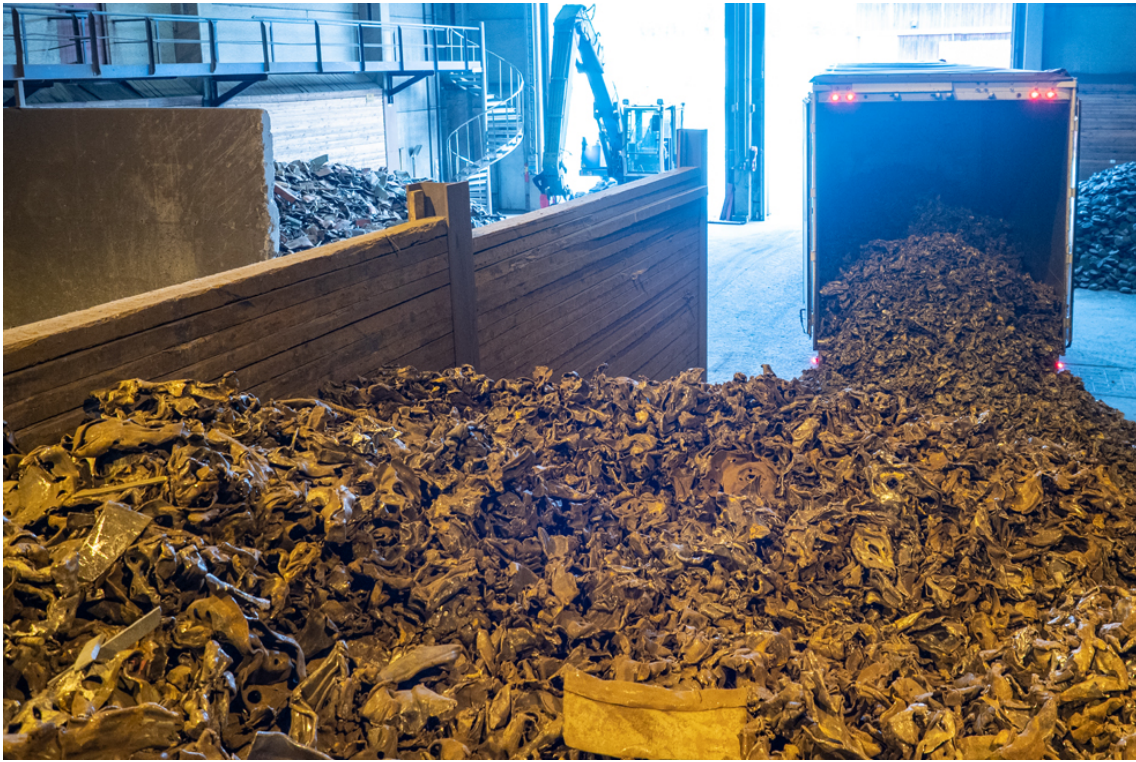
Figure A9 A scrap bin in a Norwegian iron foundry, promoted by the Auto Recycling scheme Autoretur. [239] In the background, another heap can be seen – this is pure virgin pig iron, necessary to dilute and compensate the many contaminants in the car scrap. The pig iron in the picture is produced from African beach sand. Photo Autoretur.
