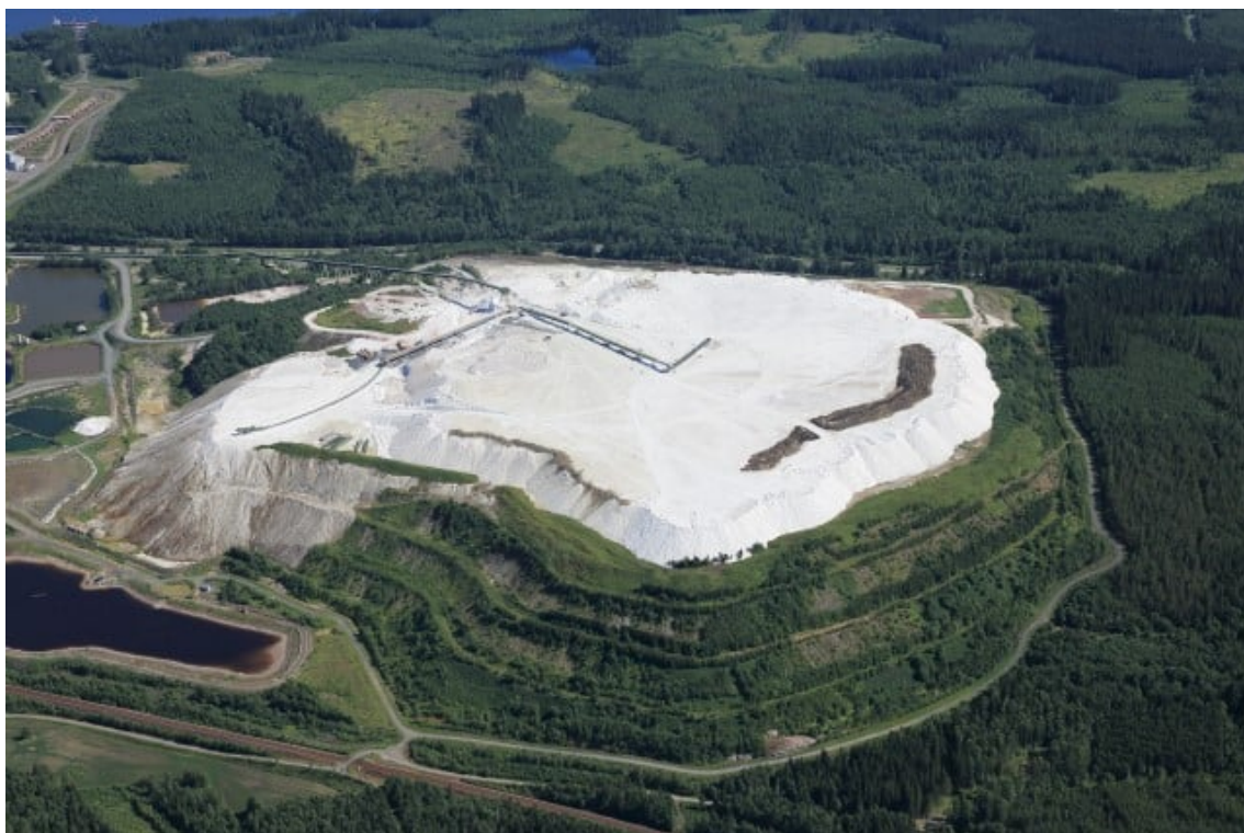
Figure A1 PG stacks in Siilinjärvi has a growing inventory of CRMs.
