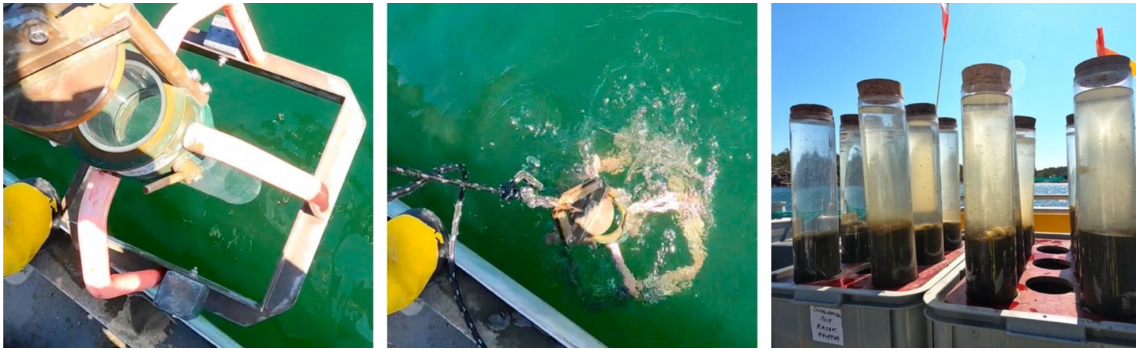
Figure 2. Photos of the sampling with the kajak tube corer from the boat in Stor fjärden, and collected sediment cores with intact bottom water overlying the sediment surface.
