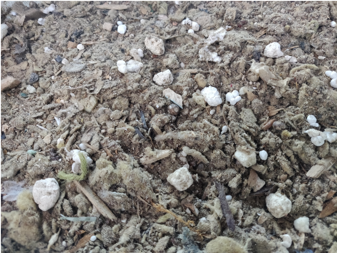
Figure 14. Example of reject from mechanical CDW separation [91] . (Source: Puhakka 2020)
