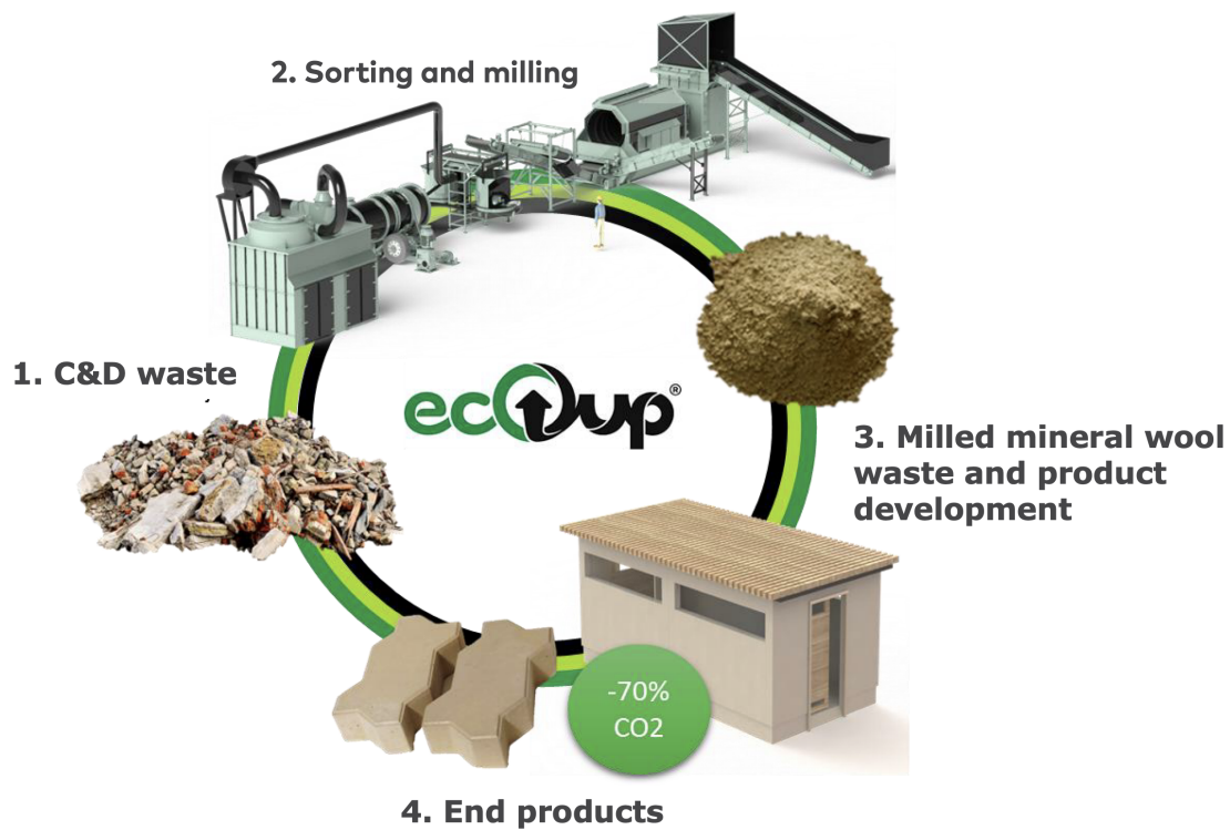
Figure 16. EcoUp concept for mineral wool recycling. (Source: EcoUp)
