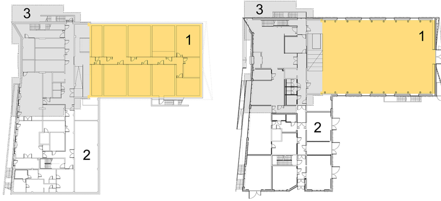
Figure 29. Basement (left) and the ground floor plan, Mäemaja building. The structures of the old test hall (1) were mainly preserved and spaces with poor functionality (3) demolished. New, larger office part (2) was constructed with a CLT timber frame.
